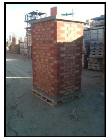
Completed tower Ready for installation
